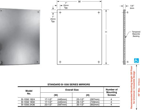
Note: Overall width and height of custom 1556-series mirrors will be 1/2" (12mm) smaller than dimension specified.
