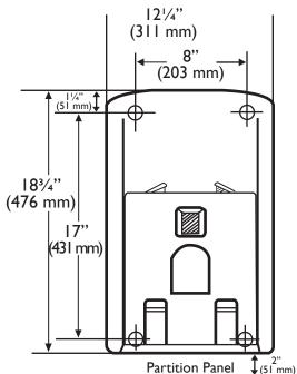
Mount 2" (51 mm) from bottom of door or 14" (356 mm) from floor
